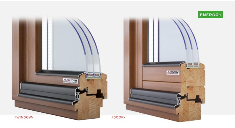
EcoTherm92 inward opening tilt and turn windows have been designed for passive housing. 92mm depth of the frame and sash provides high level of rigidity. 4-layer wood treatment perfectly protects windows from weather factors.
